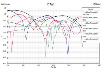
As per the above structures it is being shown that maximum return loss of -40dB is obtained when Rogers 3010 dielectric material was used. The maximum bandwidth in this regards is calculated as 25% for the same material used as substrate.
