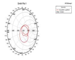
The Smith Plot in all the five mentioned cases is evaluated as distributed along the resistive line. The smith loss plot is effectively showing that VSWR is under the range of 1 to 1.5 for all the considered cases.
